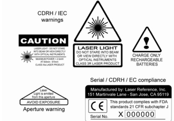
Note: The Alpha C is a CDRH class II laser and an IEC 60825 class 2 laser. It conforms to applicable EC directives regarding RFI and EMI, and to FDA performance standards 21 CFR subchapter J.
